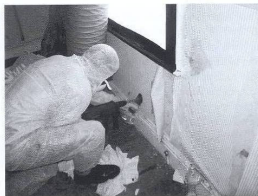
Fig. 3. Mortar sampling to determine the extent of residual moisture in the building fabric.
